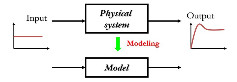
A model is used for the analysis and design of control systems.
