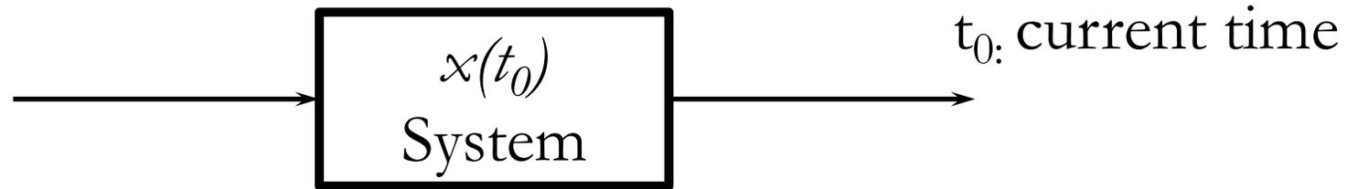
**Lumped system:** State vector is finite dimensional
