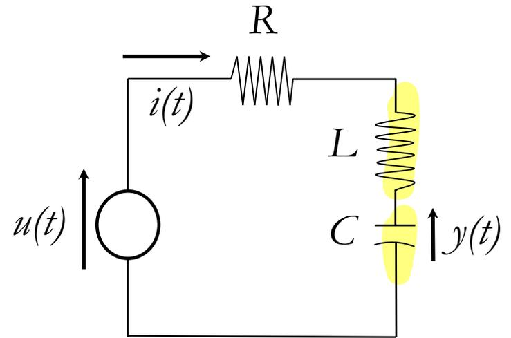
**Define State Variables** (current for inductor, voltage for capacitor):
